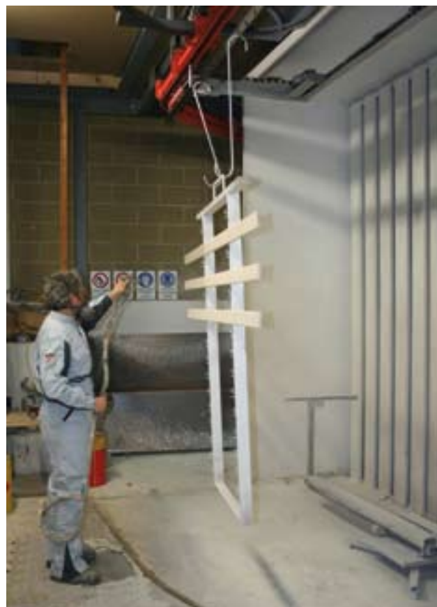
6 - The dry paint booth. See the load rotators that allow to coat easily the second side of the window frame.
